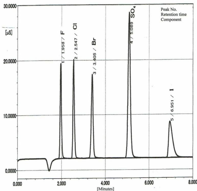
Fig. 1 Ion chromatogram; Combustion of NAC-st4
